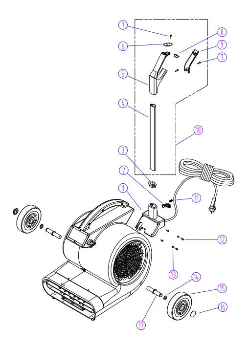
THE AXLES HAVE A VERY TIGHT TOLERANCE FIT.
