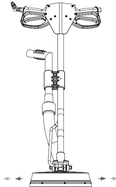
Hold the machine at waist level and use side to side.
