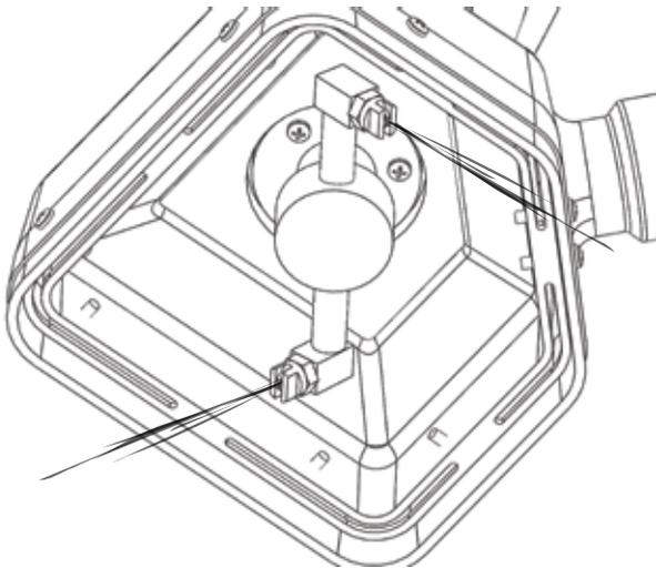
After the extractor is turned on and vacuum is engaged, squeeze the High-Pressure Trigger Gun. Liquid flows through the Solution Hose and activates the Spinner Bar.
