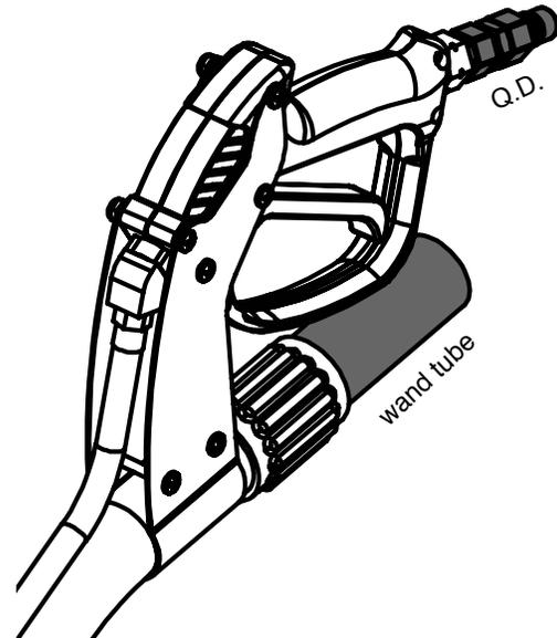
After the Vacuum Hose and Solution Hose are attached to the extractor, connect the Solution Hose to the Male Quick Disconnect, and the Vacuum Hose to wand tube.
