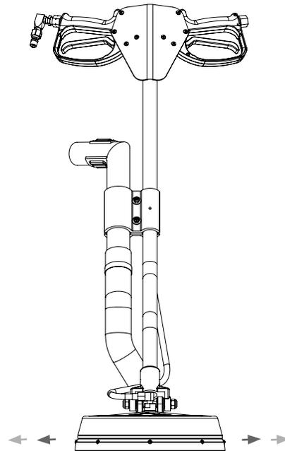
Hold the machine at waist level and use side to side.
