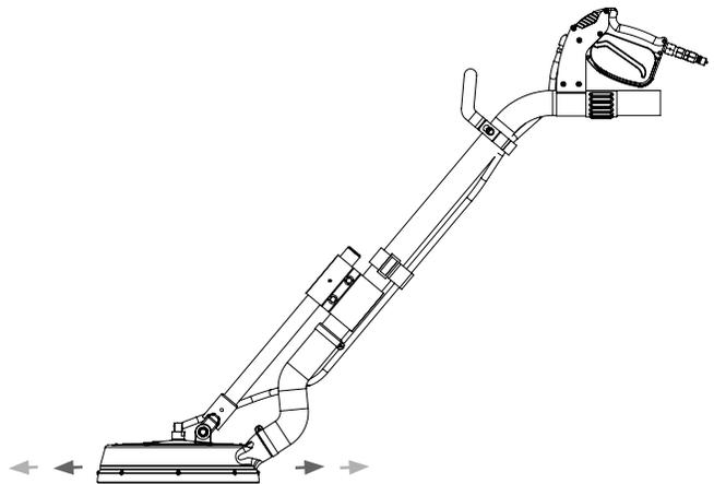
Hold the machine at waist level and use a back-and-forth motion.
