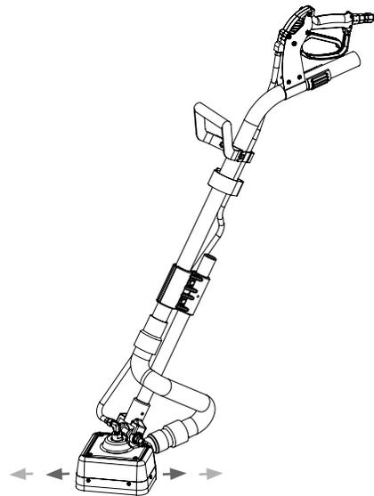
Hold the machine at waist level and use a back-and-forth motion.
