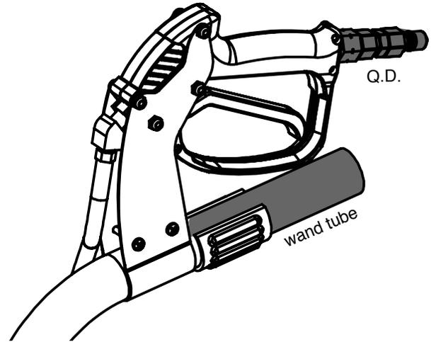
After the Vacuum Hose and Solution Hose are attached to the extractor, connect the Solution Hose to the Male Quick Disconnect, and the Vacuum Hose to wand tube.
