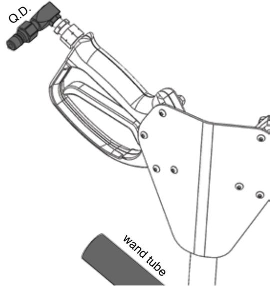
After the Vacuum Hose and Solution Hose are attached to the extractor, connect the Solution Hose to the Male Quick Disconnect, and the Vacuum Hose to wand tube.
