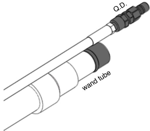
After the Vacuum Hose and Solution Hose are attached to the extractor, connect the Solution Hose to the Male Quick Disconnect, and the Vacuum Hose to wand tube.
