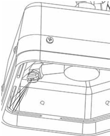
After the extractor is turned on and vacuum is engaged, squeeze the High-Pressure Trigger Gun. Liquid flows through the Solution Hose and activates the Spinner Bar.
