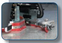
The swinging squeegee (on disc models) is uniquely designed for 100% water pick up, even in turns.
