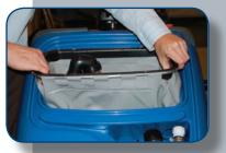
The bag is easily removed without tools for cleaning, providing improved hygiene.
