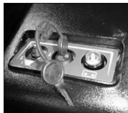
The brush control switch, key-start, and battery level meter are conveniently located next to the seat.
