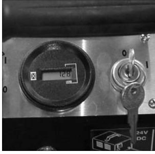
The Wrangler 2016 is available with a Key-And-Hour-Meter option. The key increases safety, preventing unauthorized operation. The Hour Meter makes it easy to track runtimes for routine maintenance procedures.
